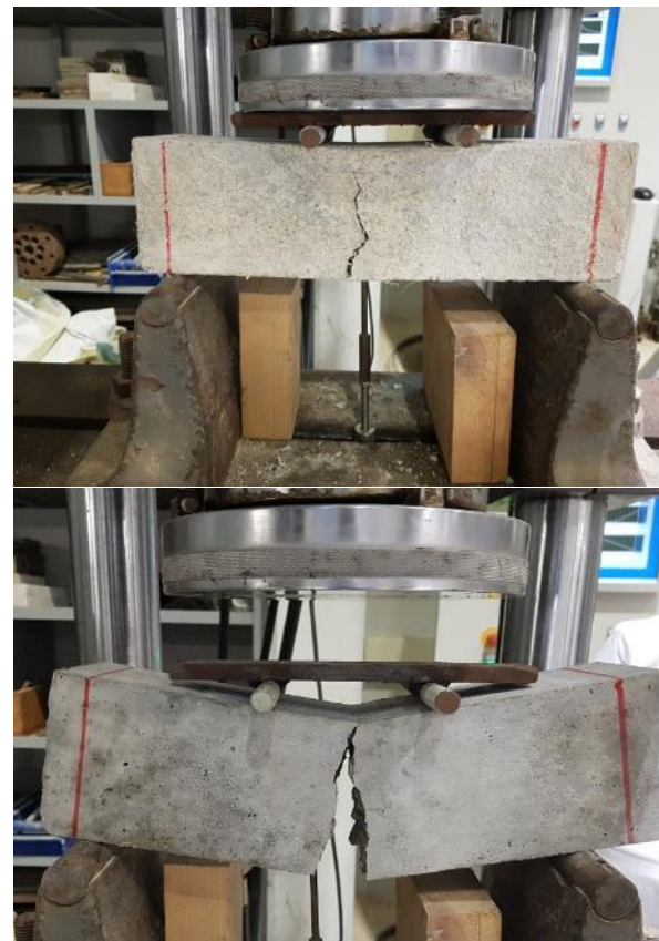
Fig. 3: State after rupture with fibers (top), without fibers (bottom)
