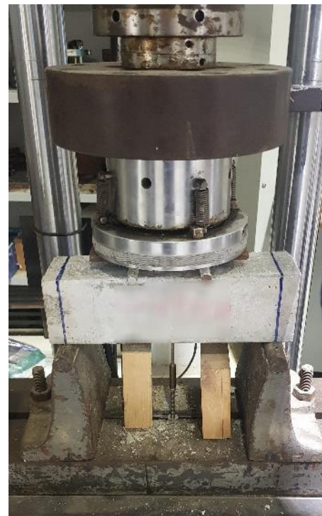
Fig. 1: Flexural strength test setup
