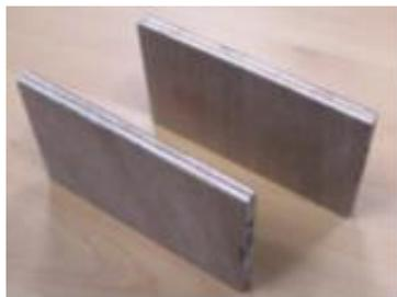
Fig. 92: The wooden boards (70x110x7 mm) tested according to ASTM C-1114:06.
