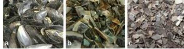
Fig. 86: Mussel shell used: a) whole shell (S), b) mussel shell gravel (MG), and c) coarse mussel shell sand (CMS).
