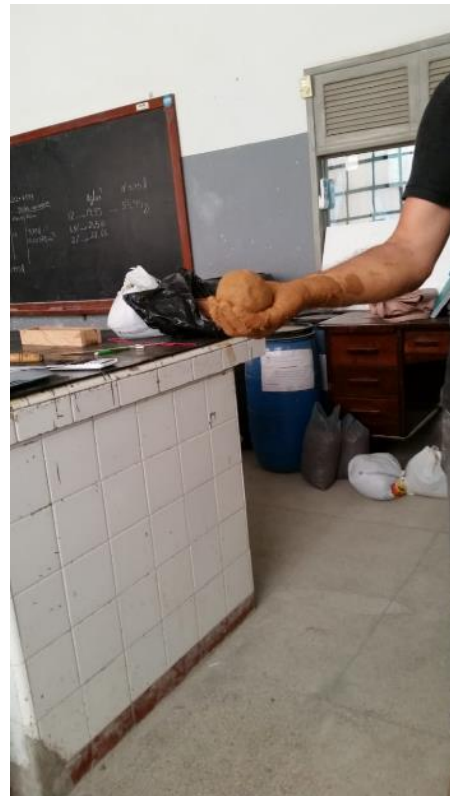
Fig. 3: Technique for estimation of suitable water content (Falling Ball test).
