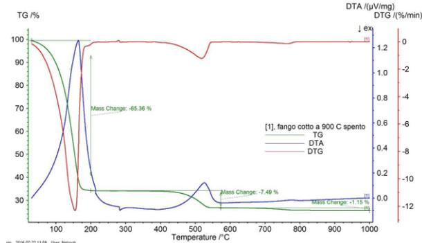
Fig. 1. STA of slaked lime obtained by marble slurry.
