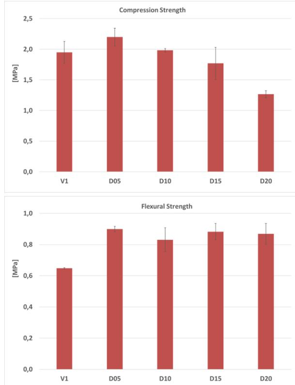
Fig. 9: Compression and flexural strength for mortars prepared with or without diss fibers, after three months of hardening.
