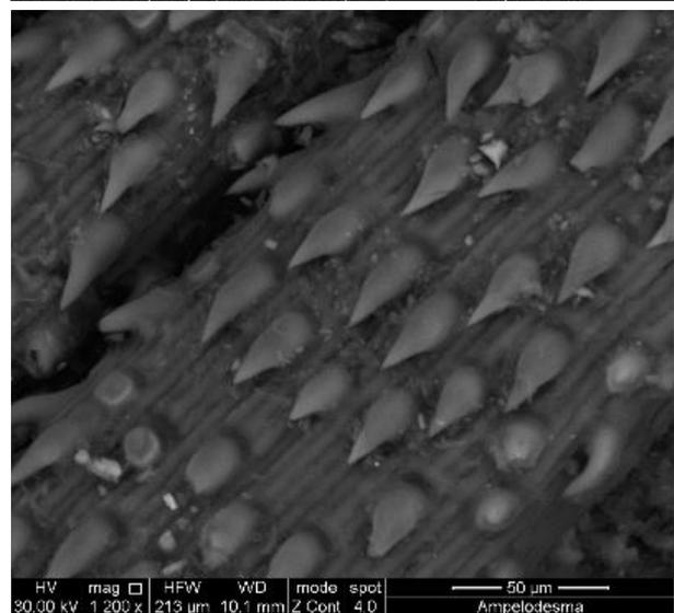
Fig 3 Diss fibers as observed in Secondary electron modes in SEM.
