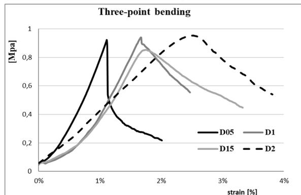
Fig. 10: Three point bending stress strain curves for mortars prepared with or without diss fibers, after three months of hardening.
