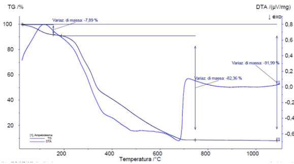
Fig.5: STA on diss fiber, note that total mass loss is equal to 92% including 7.89% of humidity.
