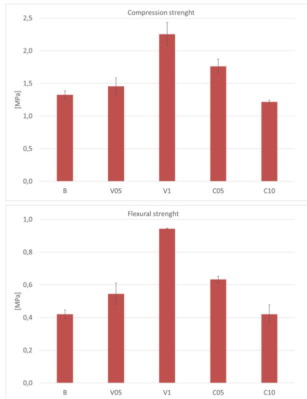
Fig. 8: Compression and flexural strength for mortars prepared with or without diss ashes, after three months of hardening.
