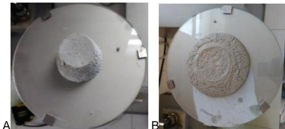
Fig. 7: mortar on flow table before, A, and after, B, workability test.
