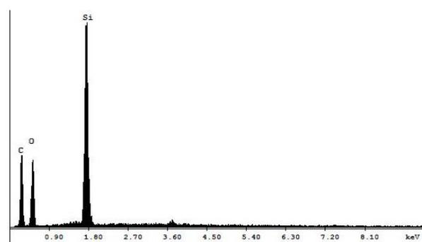
Fig 4 EDS analysis of hooks visible on the diss fibers surface.
