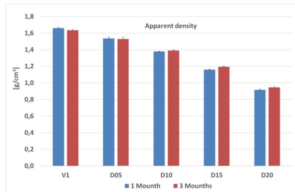
Fig. 10: Apparent density of mortars prepared with or without diss fibers, after one or three months of hardening.
