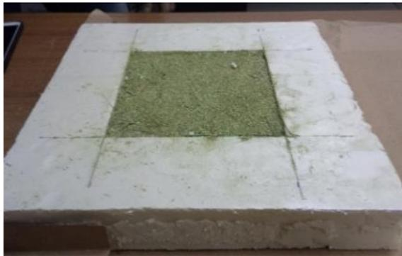
Fig.6: Polystyrene mould filled with diss fiber for thermal conductivity measurements.
