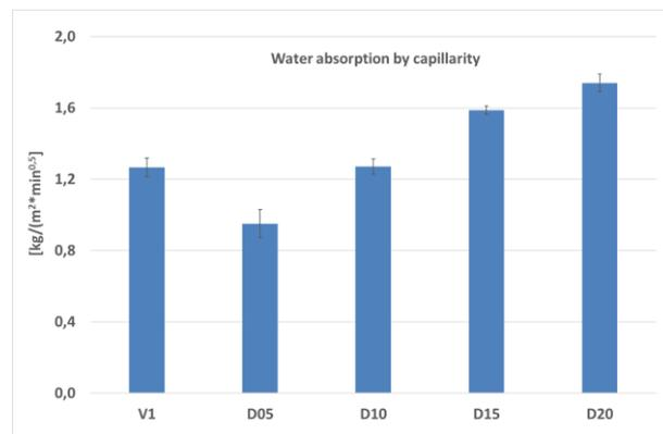
Fig. 11: Water absorption for mortars prepared with or without diss fibers, after three months of hardening.
