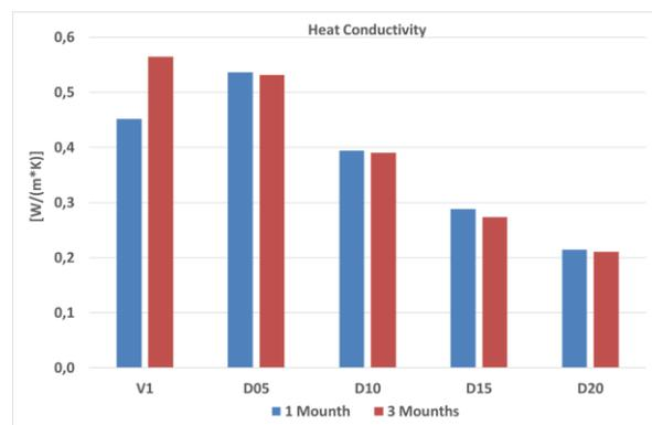
Fig. 12: Heat conductivity for mortars prepared with or without diss fibers, after one and three months of hardening.
