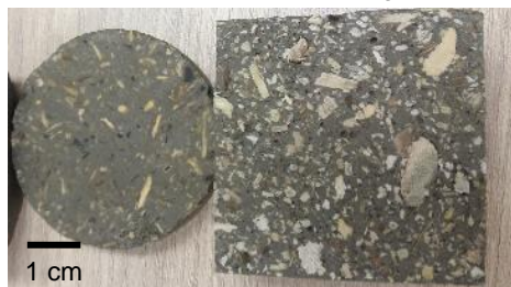
Fig. 6: Homogeneity of bio-concretes. Top view (left) and tangential section (right) of one of the specimens.
