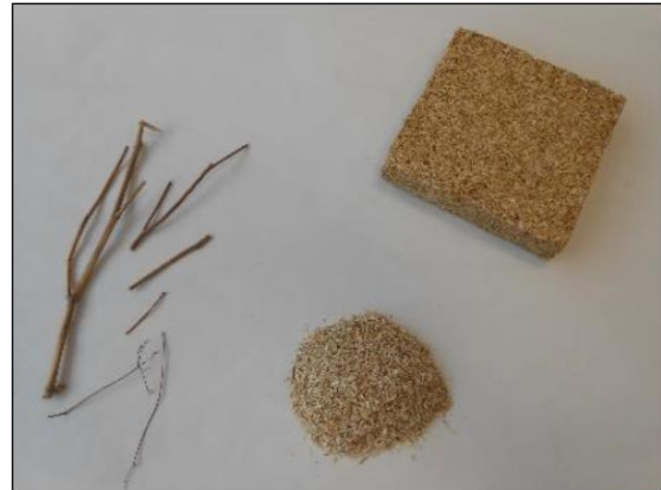
Fig. 4: Photograph of raw straw, milled straw and insulation block from the latter (from left to right).
