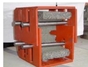
Fig. 2: Tensile test of a strut from a shuttering block
