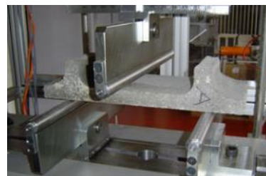
Fig. 3: Flexural test of a face from a shuttering block
