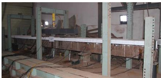
Fig.9. Test of glulam and concrete composite beams
