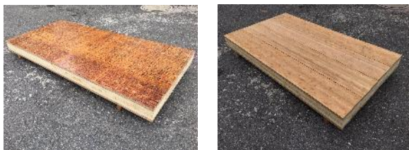
(a) CLBT with thin-strip glubam as surfaces (b) CLBT with thick-strip glubam as surfaces Fig.2. CLBT with different glubam outer layers
