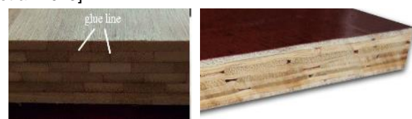
(a) Glubam made from thick bamboo strips (b) Glubam made from thin bamboo strips
