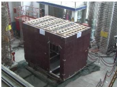
Fig.6. Shake table testing of full-scale glulam shear wall room model.
