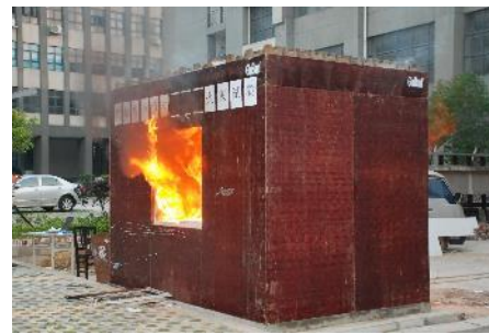
Fig.13. Fire testing of a full-scale glubam room model
