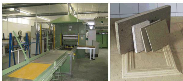
Fig. 5: Heating press and selected product samples
