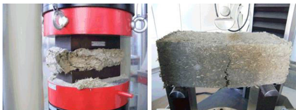
Fig. 11: Test setups for the characterization of block specimens based on mineral bond wet preserved hemp fibres
