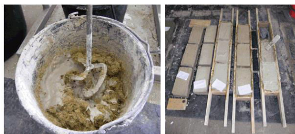
Fig. 6: Component mixing and forming of test blocks
