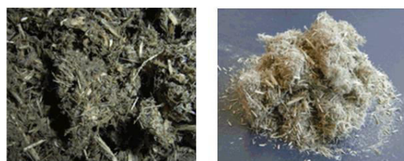
Fig. 4: Wet extruded fibre material (left) and dried fibre material after milling and drying (right)
