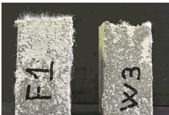
Fig. 8: F specimen (on the left) and W specimen (on the right) after bending tests.
