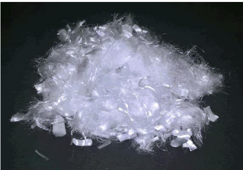
Fig. 2: Polypropylene fibers used to reinforce mortars.
