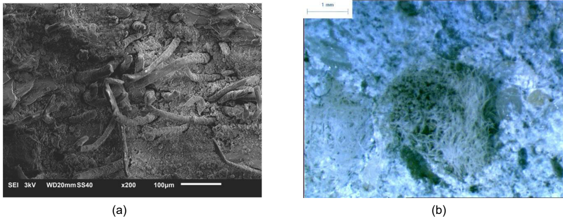
Fig. 5: Characteristic part of the W specimen (not stored in water) with visible bunches of the wool filaments: (a) SEM observation, scale bar =100 µm, (b) stereomicroscope, reflected light, scale bar =1000 µm
