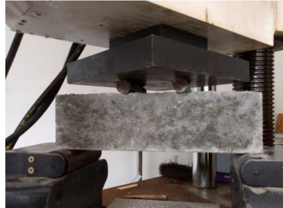
Fig. 2 : Testing Beam specimens for flexural strength.
