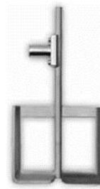
Fig. 7: Wing stirrer called cement paste probe V0013.
