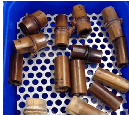
Fig. 4: Set 5 - specimens less attacked by mold.
