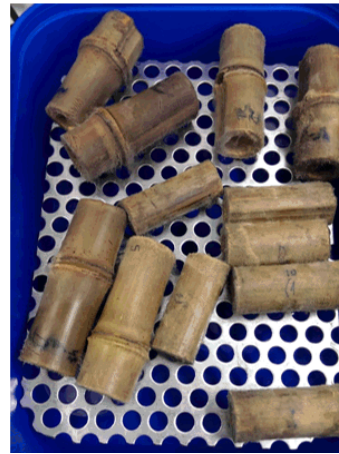
Fig. 3: Set 1- specimens attacked by mold
