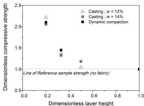
Fig. 7: Dimensionless compressive strength of fabric reinforced samples versus the dimensionless height of layers of earth-based materials.
