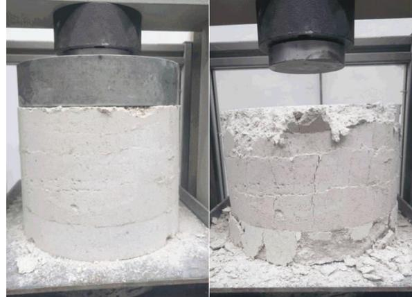
Fig. 8: Observation of the dynamically compacted samples with 4 woven fabrics before and after the compressive strength measurement.
