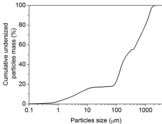
Fig. 3: Particles size distribution of the powders
