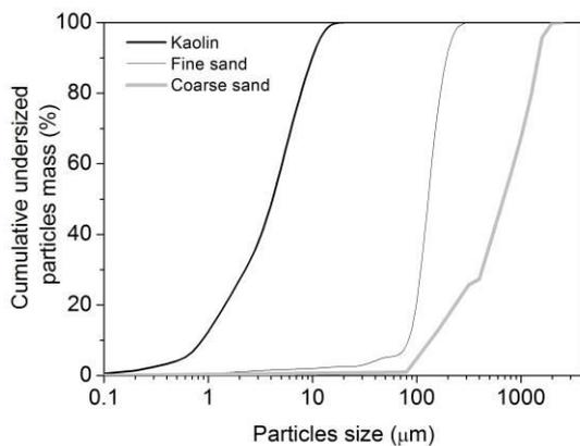
Fig. 1: Particles size distribution of the powders
