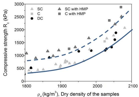
Fig. 6: Evolution of the compressive strength of the sample after drying versus the dry density for the different forming processes and possible use of HMP.
