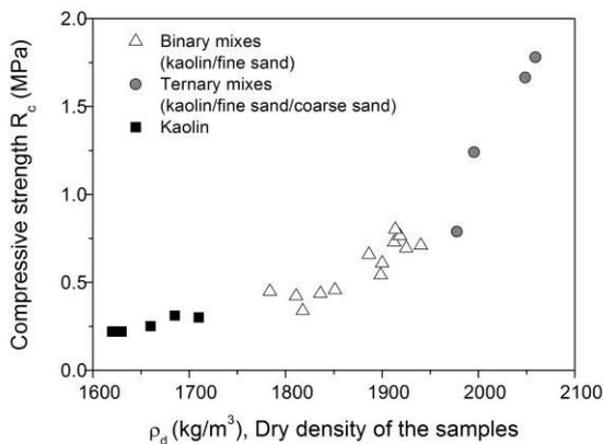
Fig. 4: Compressive strength as a function of dry density for kaolin, binary mix (fine sand+kaolin) and ternary mix (coarse sand+fine sand+kaolin)
