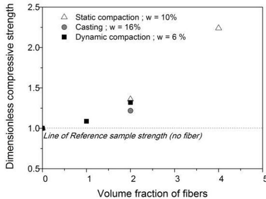
Fig. 9: Dimensionless compressive strength of fiber reinforced samples versus the volume fraction of fibers contained in earth-based materials.
