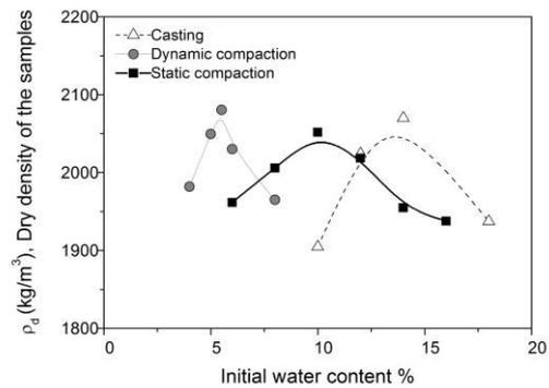
Fig. 5: Influence of the initial water content (water added during mixing) on the dry density of the samples for the 3 tested forming process. The static compaction was performed at a maximum load of 25 MPa.
