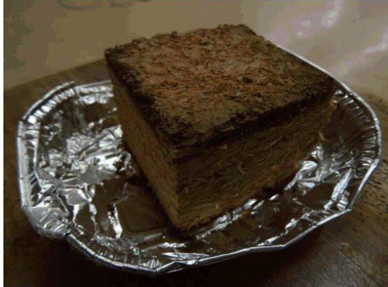
Fig. 4: S6 sample after ignition time test
