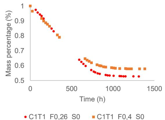
Fig 5. Drying curves of formulas with hemp shiv on dry sieved earth and sand ratio variation
