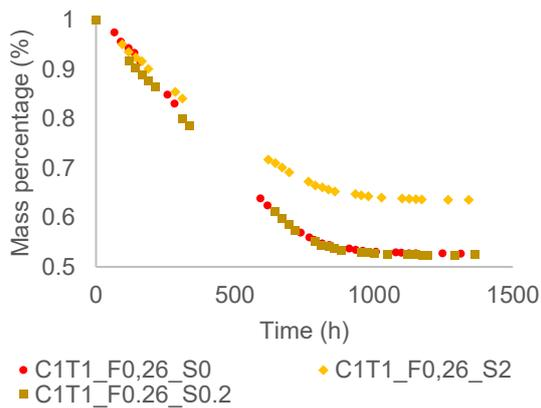
Fig. 6. Drying curves with sand on dry sieved earth ratio variations
