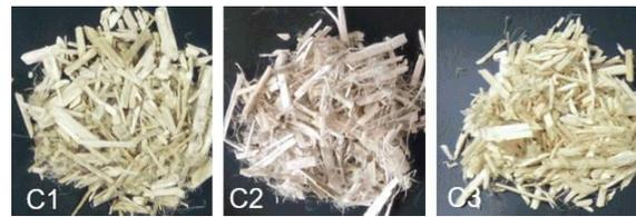
Fig 1. Samples of hemp shives: C1 and C2 are hemp shives from a local hemp producer, C3 was bought in a convention construction shop.
