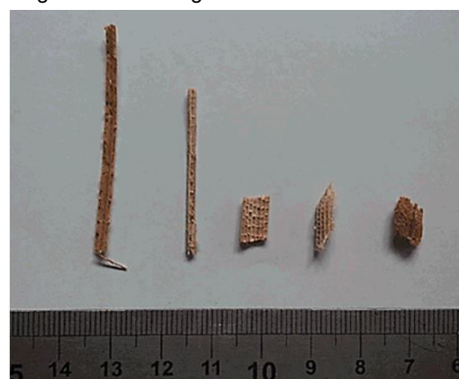
Figure 21 : Morphology of the transverse fraction of Typha
