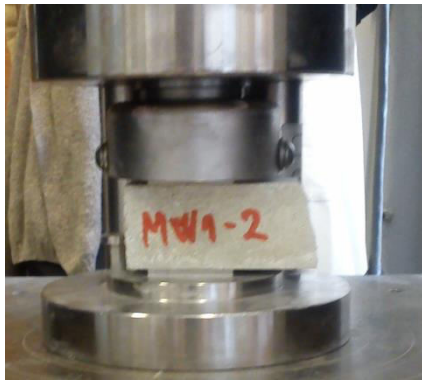
Fig. 2: Three-point bending test and compression test.
