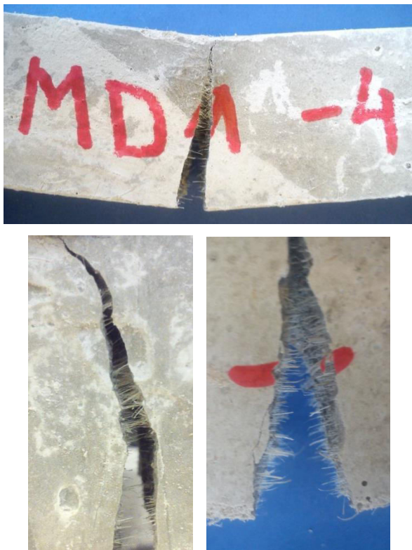
Fig. 6: Fibres bridging across the crack.
