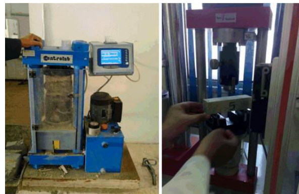
Fig.2: Compressive strength test (Left), flexural strength (Right).
