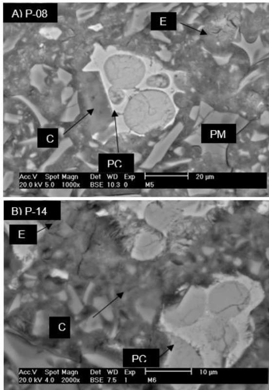
Fig. 17 : SEM microstructures of the systems A) P-08 and B) P-14 at 28 days. (PM= pumice; C= matrix hydration products CSH; CP= Portland cement; E= ettringite).
