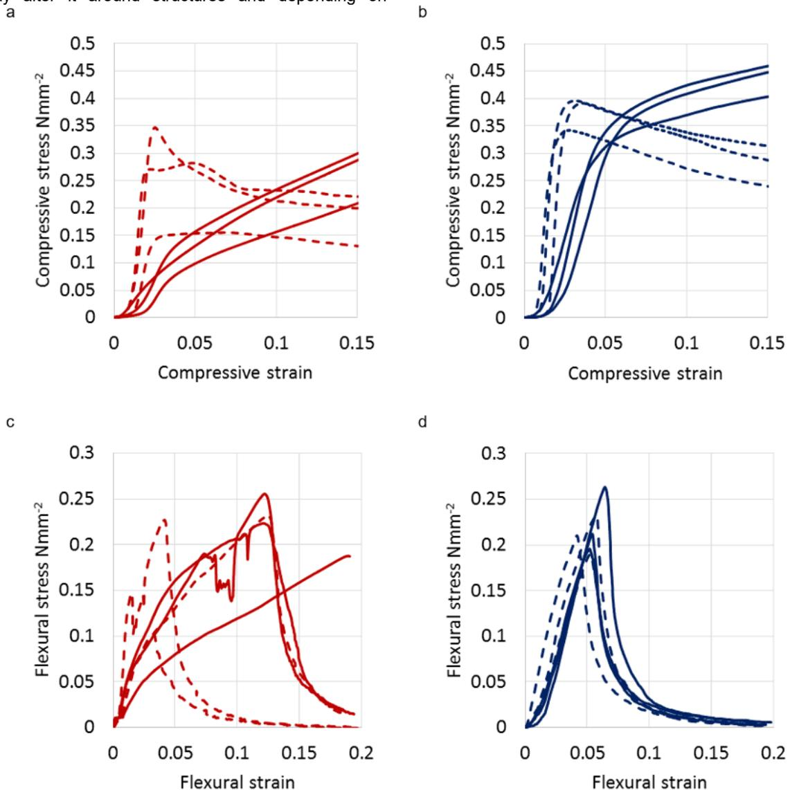
Fig. 3: Compressive and flexural stress/strain plots for hemp lime specimens produced by projection (red, a and c) and casting (blue b and d) with loading applied in the parallel direction (solid line) and perpendicular direction (dashed line).
