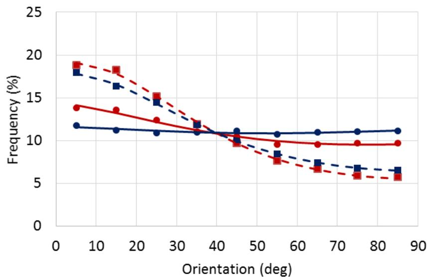
Fig. 6: The frequency distribution of hemp particles in planes viewed in the parallel (solid line) and perpendicular (dotted line) directions, and formed by projection (red) and casting (blue).
