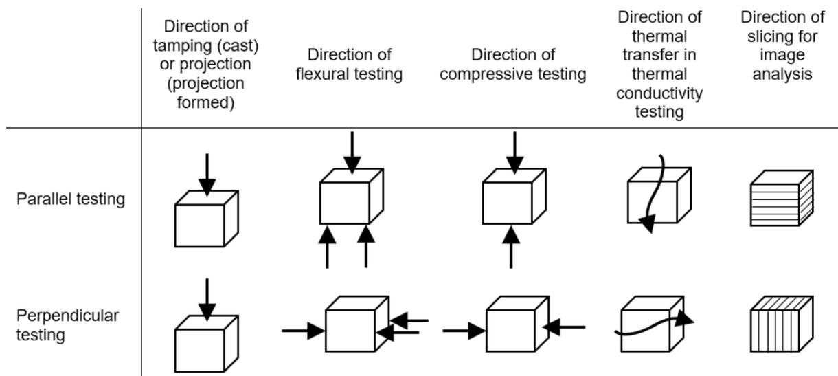
Fig. 2: The casting and loading arrangements for parallel and perpendicular loading.
