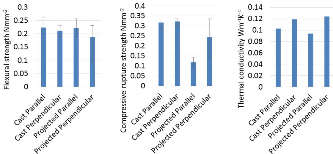
Fig. 5: The directional peak flexural strength, compressive rupture strength and thermal conductivity of projection formed and cast hemp-lime.
