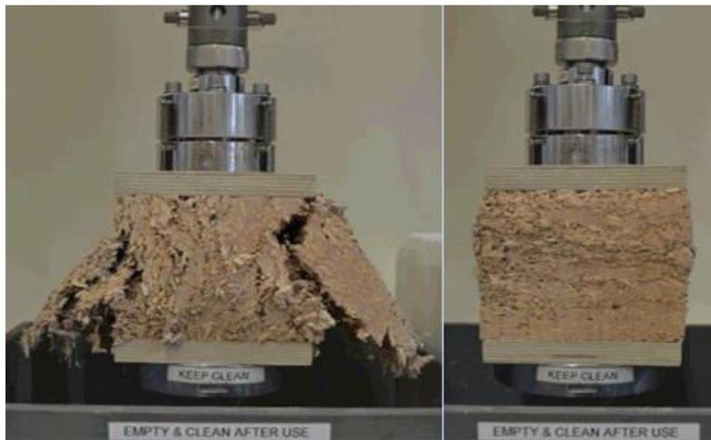
Fig. 4: Typical compressive failure modes of hemp-lime loaded in the perpendicular and parallel directions, left and right respectively.
