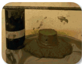
Fig. 4: Slump of cylinder test
