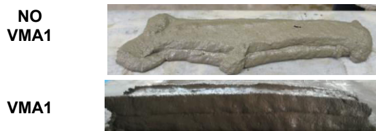
Fig. 11: Effect of VMA1 on shape of 2 printed layers
