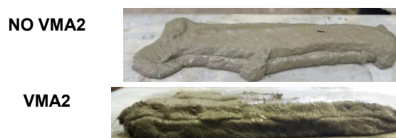
Fig. 13: Effect of VMA2 printed layers
