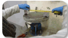
Fig. 2: Slump flow test
