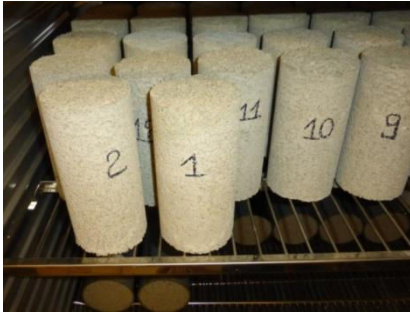
Fig. 5 : Plant-based concretes during the curing period Preparation of specimens
