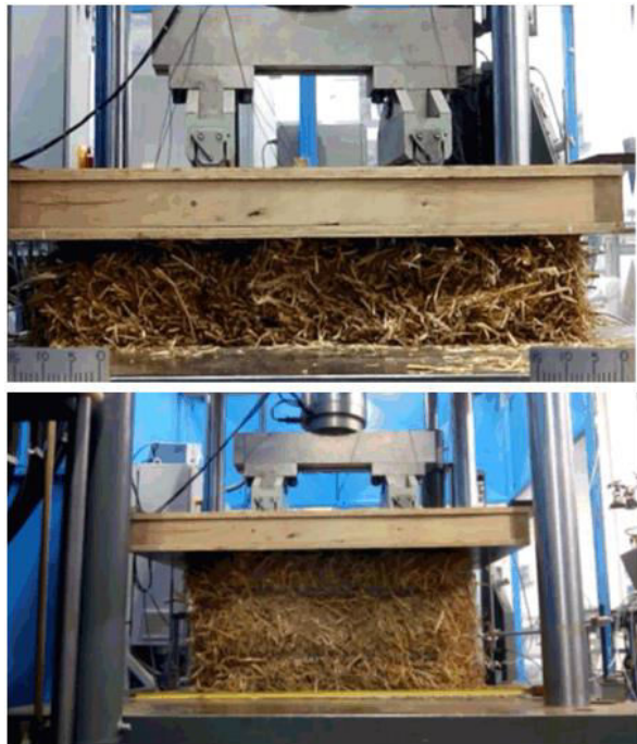
Figure 4: The compression device and the two different configurations. (bottom) edge, at the beginning of a test; (top) flat, with a strain of 0.77
