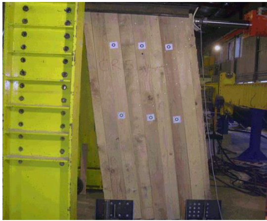
Fig 7: Timber cross plank wall in test.
