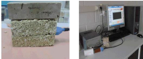
Fig. 4: Hot wire NEOTIM FP2C conductivity meter with SP sample
