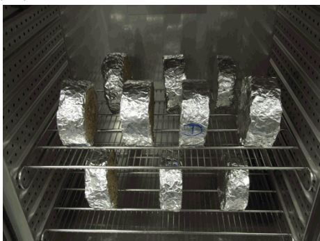
Fig. 5: Samples in Binder KBF climatic chamber
