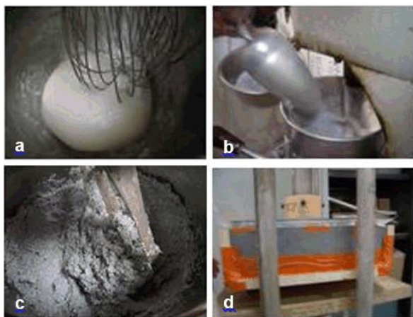
Fig. 5: Production process: a) Binder mixing; b) Addition of the load; c) Mixing; d) Compaction.
