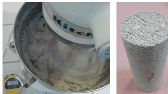
Fig. 25: Production process: Foaming process and Mineral foam sample.
