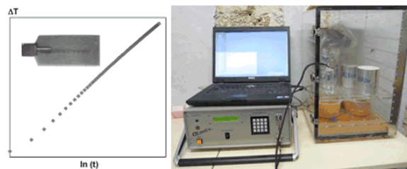
Fig. 23). In this study, the power used ranges between 0.205 and 0.378 W and the heating time is 120 s. The thermal conductivity of a pair of specimens is the average of five values with a variation coefficient lower than 5 %. The thermal conductivity of one material is the average value of all measurements.
