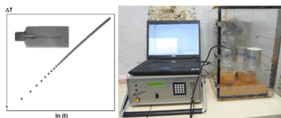
Fig. 23: Measurement of thermal conductivity at dry state left: experimental thermogram, right: CT meter, hot wire and dry chamber.
