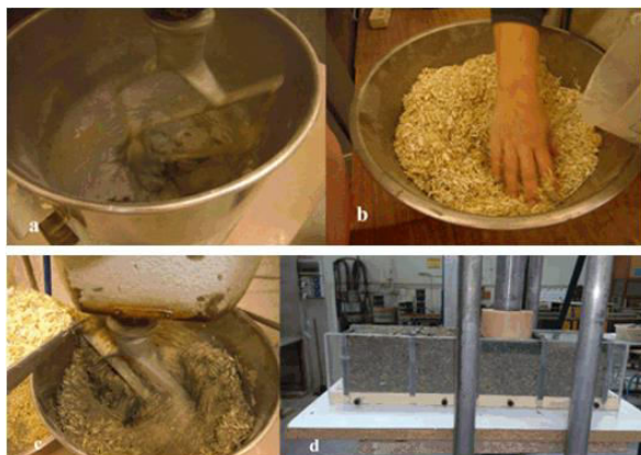
Fig. 24: Production process: a) Binder mixing; b) Hemp mixing by hand; c) Addition of the moist hemp and mixing; d) Compaction.
