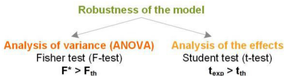
Fig. 37 : Flow chart of statistical analysis for defining the robustness of the model
