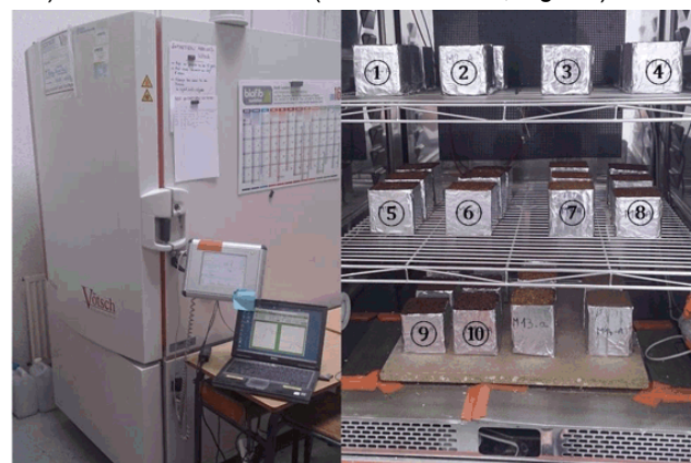
Fig. 41: Experimental device for the measurement of Moisture Buffer Value
