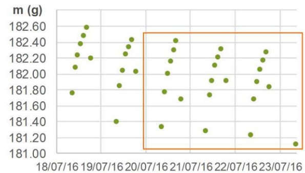
Fig. 47: Moisture uptake and release for sample n°1-A
