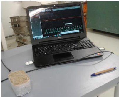
Fig.2: The experimental device for evaluating moisture buffering of DPFC.
