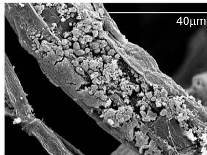
Fig. 60 SEM picture of kraft pulp in PC submitted to 4 wet/dry cycle.
