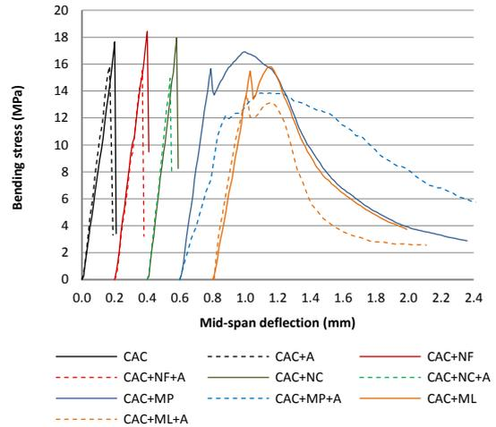
Fig. 55 Representative curves obtained from the bending test. The curves were displaced 0.2 mm respectively to avoid the results overlapping.
