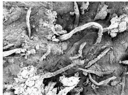
Fig. 61 SEM image of CAC+MP matrix after wet/dry cycles.
