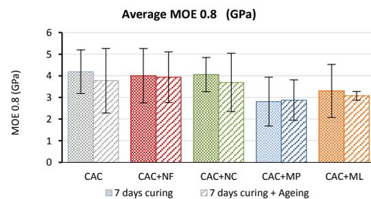
Fig. 57 Average values and standard deviation of MOE 0.8 obtained from bending tests
