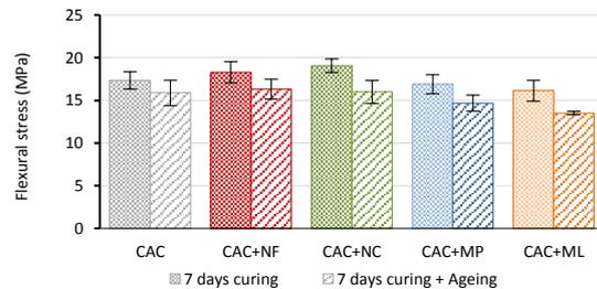
Fig. 56 Average values and standard deviation of MOR obtained from bending tests.
