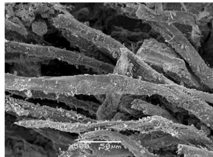
Fig. 62 Microstructure of fiber surfaces of CAC+MP matrix after wet/dry cycles.
