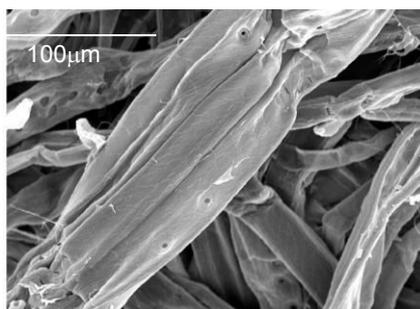
Fig. 59 SEM picture of Kraft pulp fibers.
