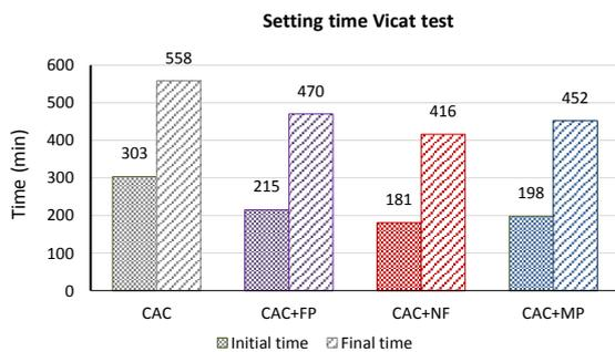
Fig. 54 Setting times for Vicat test
