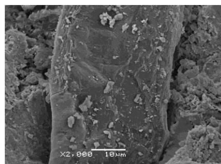
Fig. 63 Microstructure detail of fibers in sample CAC+MP after the wet/dry cycles.
