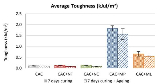
Fig. 58 Average values and standard deviation of toughness obtained from bending tests
