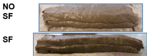
Fig. 8: Photos of layers made with and without SF
