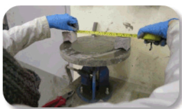
Fig. 2: Slump flow test
