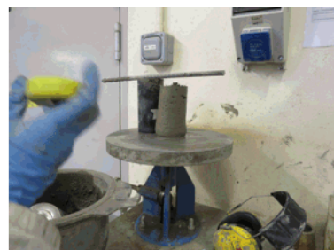
Fig. 4: Slump of cylinder test
