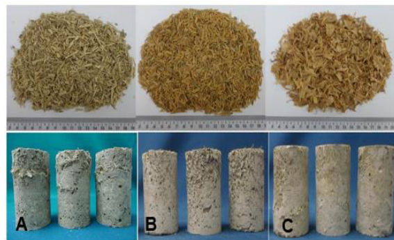
Fig. 1: Raw biomass and samples of the equivalent bio-based composites of (A) bamboo particles, (B) rice husk and (C) wood shavings
