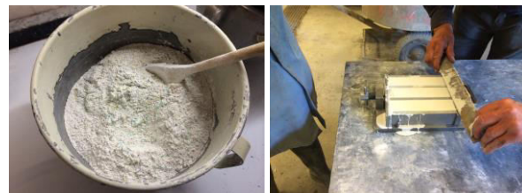
Fig. 70. Mixing and casting of prisms and cylinders
