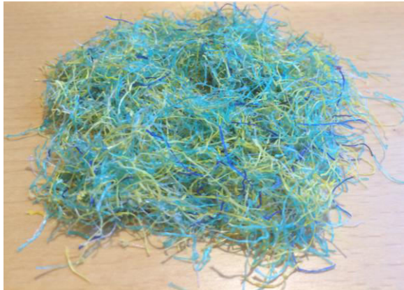
Fig. 68. Monofilament fibres of polyethylene by Plastix A/S produced by mechanical cutting operation
