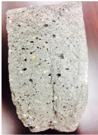
Fig.3: Voids introduced in mortar mix with 8% cement replaced by biochar
