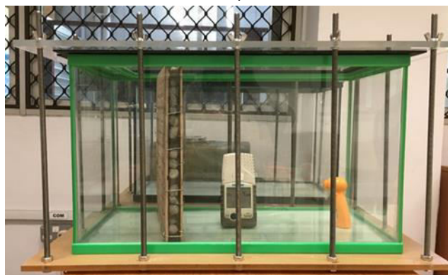
Fig. 1. Basic experimental setup for studying different types of pellets. In this case, only the carbon dioxide analyzer (Telaire 7001) was shown.
