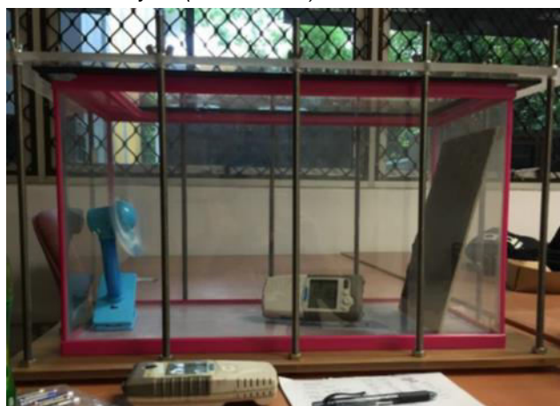
Fig. 2. Basic experimental setup for studying different types of plaster. In this case, only the carbon dioxide analyzer (Telaire 7001) was shown.
