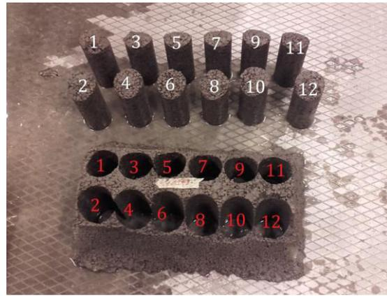
**Figure 2: Test specimens drilled from the LWA concrete block.**
