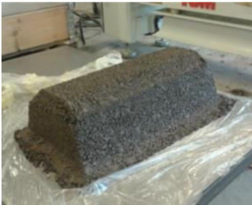
**Figure 1: a new-cast LWA concrete block.**
