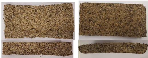
Figure 60: Photos of the dried samples in (left) ventilated furnace with pierced mold, (right):
