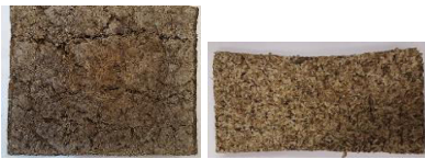
Figure 61: The photos of the dried samples in (right) ventilated oven with mold not drilled 20x10x5 cm, (left) oven 100 C with 20x20x5 cm.
