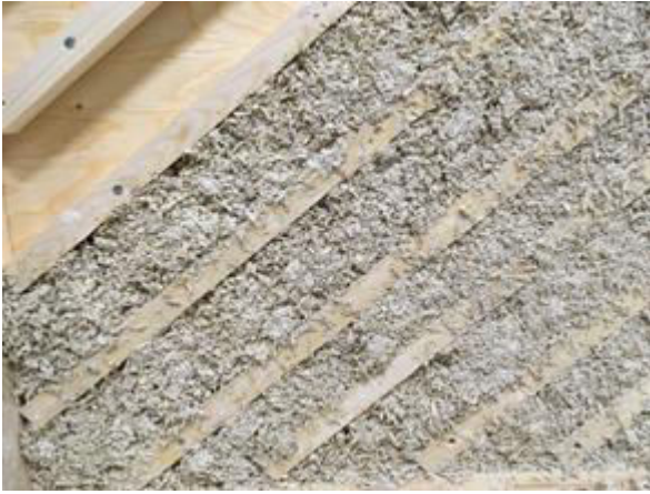
Figure 6. Testing workability of lime-hemp in between wooden slats in the lab.
