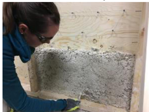
Figure 5. Testing adhesion and workability of lime-hemp in the lab.
