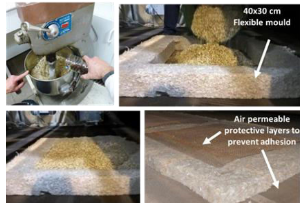
Fig. 65: Mat forming on the conveyor belt
