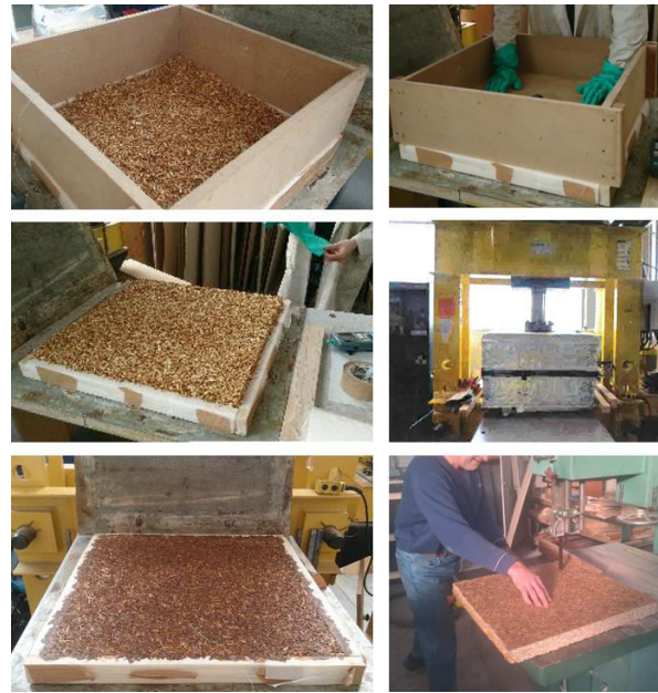
Fig. 68: Mat forming, pressing and cutting of thermopressed panels
