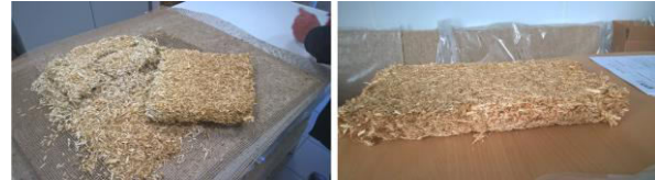
Fig. 73: Hemp shiv/Acrodur® composite manufactured using Cavac oven. (On the left, without the pre-pressing step. On the right, with the pre-pressing step)
