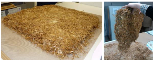
Fig. 72: Wheat straw panel after thermal treatment
