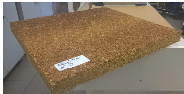
Fig. 74: Bio based insulation panel manufactured using the thermopressing process
