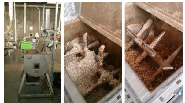
Fig. 67: Imal Pal laboratory blender with spraying nozzles
