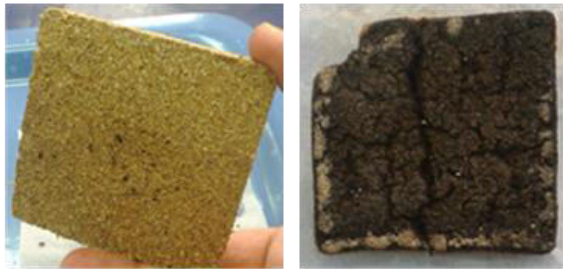
Figure 6. Specimen before and after the fire test.
