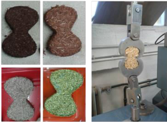
Figure 2. "8-shaped" specimens (left) used for the mechanical test evaluation (right).
