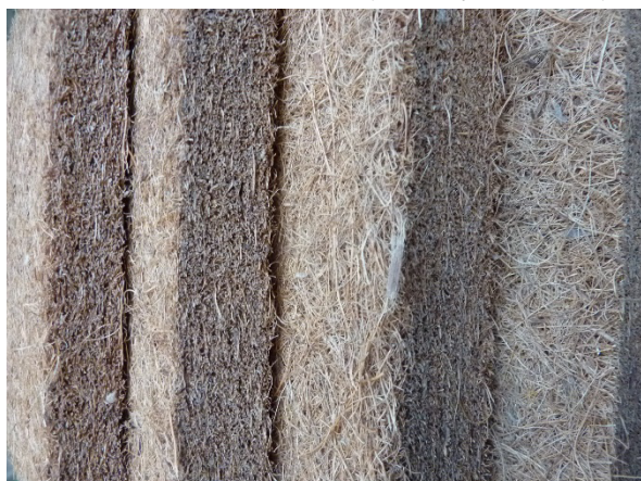
Fig. 7: Coir mats are extremely well suited for the insulation of the floorings, but also quite an interesting possibility for wall and roof constructions
