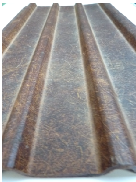
Fig. 5: Corrugated coir ply (phenol resin bonded coir) as roofing material in India
