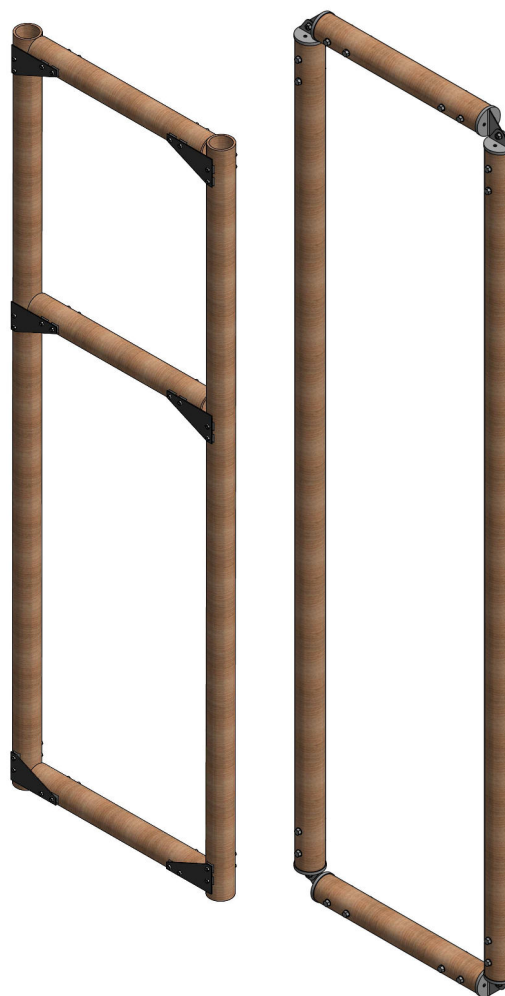
Fig. 3: Proposed Panels. Left: Gusset plate connectors with bolts and preload washers, Right: Bolted connections based on metal plates.
