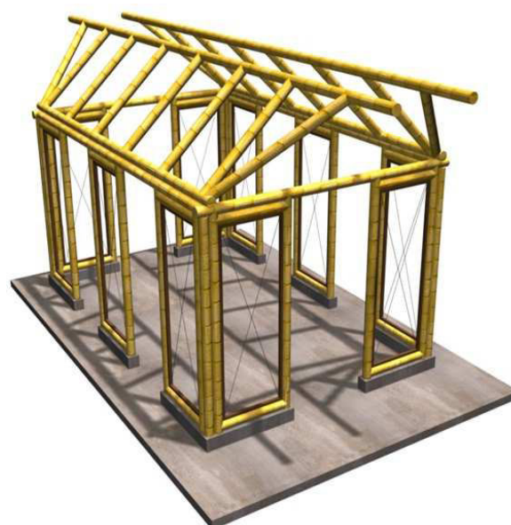
Fig. 1: Example of a GA house structure built with prefabricated panels.
