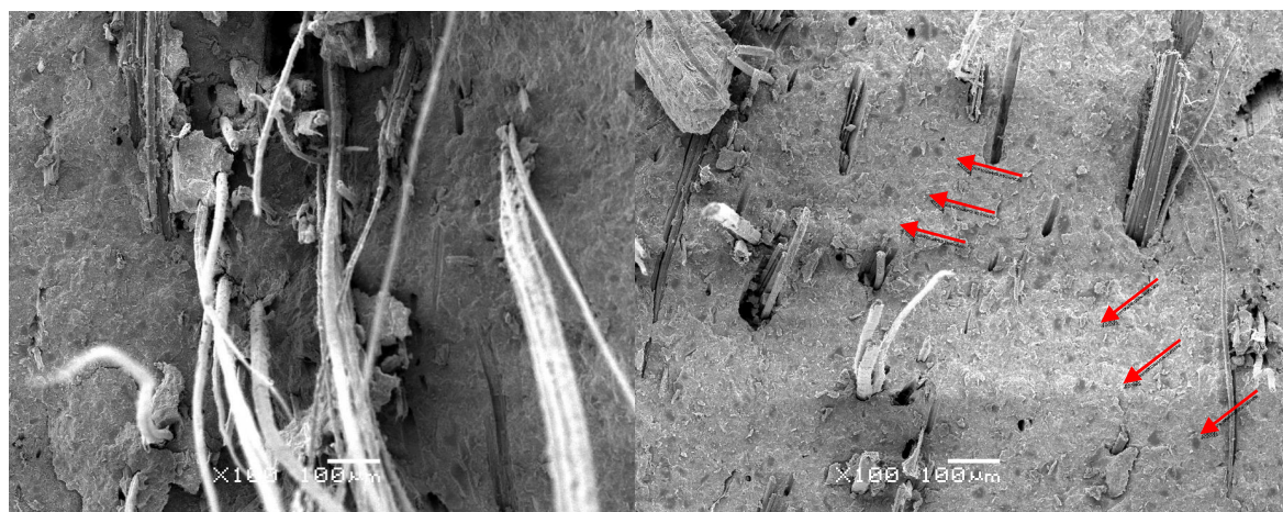
Fig.3: SEM Images of fracture surface of the unaged composite (a) and the composite aged with 25 wet/dry cycles (The arrows indicate fibres cut near the surface).
