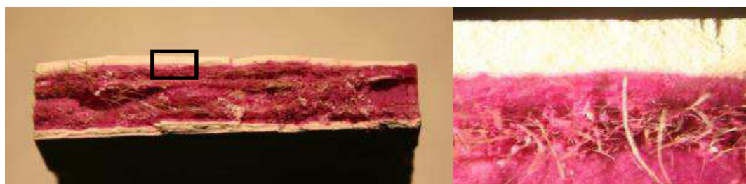
Fig.5: Picture of the fracture surface of the composite aged with 60 days outdoor exposition sprayed with phenolphthalein
