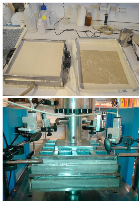
Fig. 1: Pictures of moulding procedure: laminating process (top) and compression step (bottom)
