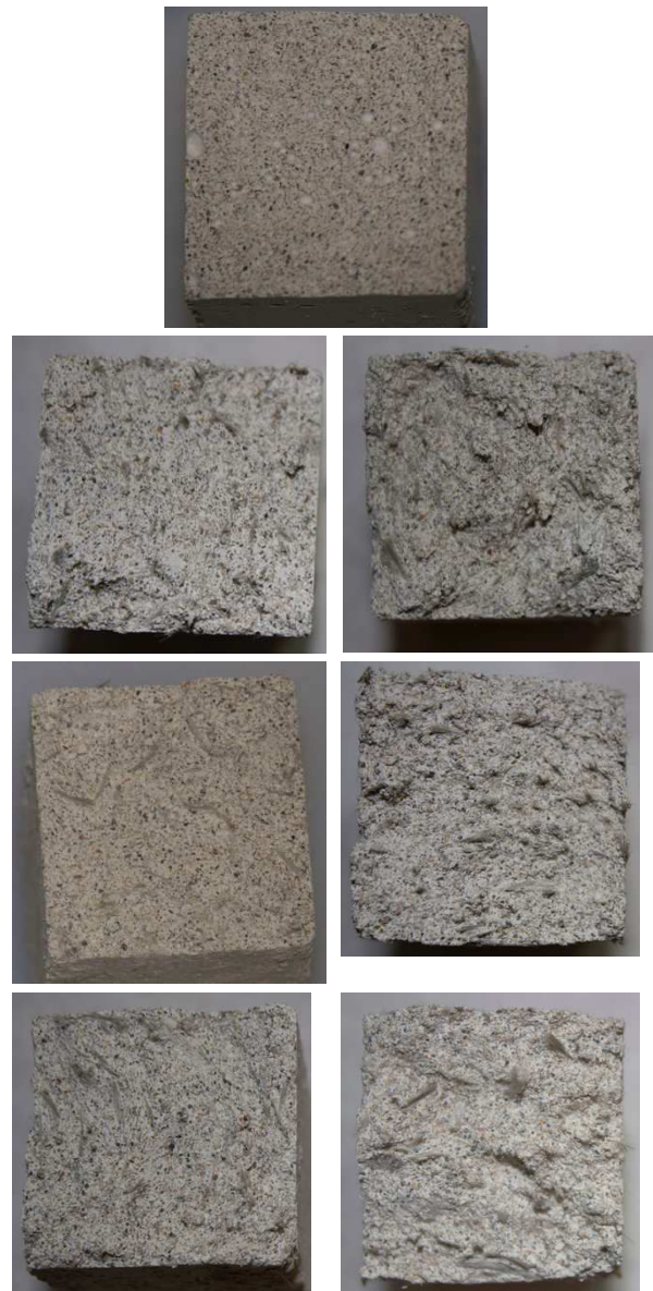
Fig. 1: Fractured surfaces of the various types of specimens a) REF; b) CH 1% siz.1; c) CH. 2% siz. 1; d)CH. 1% siz.2; e)CH. 2% siz. 2; f) CH. 1% siz.3; g) CH. 2% siz. 3)
