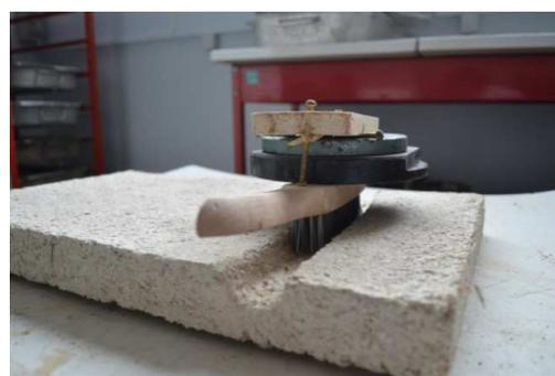
Pict. 5: abrasion test on a plaster slab
