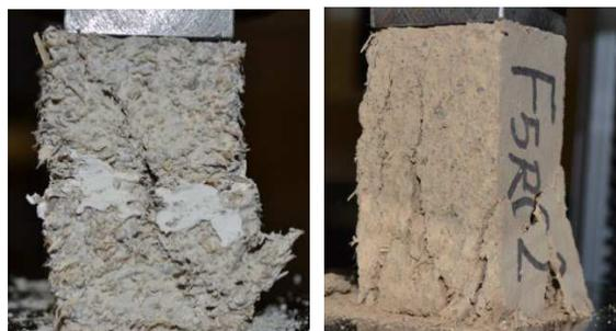
Pict 8: compressive test, F1 perpendicular and F5 parallel direction
