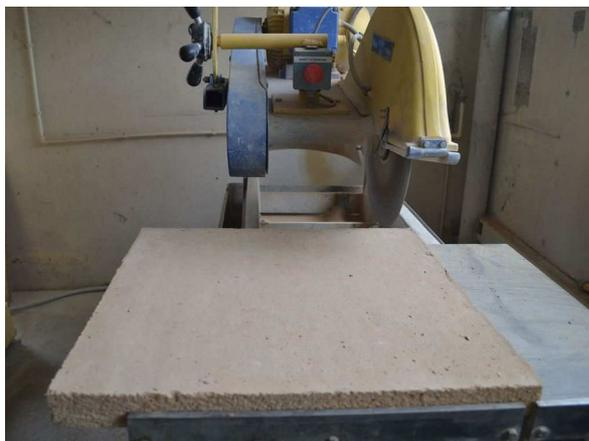
Pict. 2: sawing of a plaster slab
