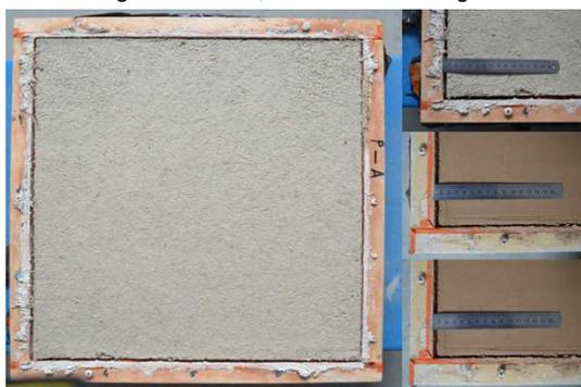
Pict. 4: shrinkage of a plaster slab
