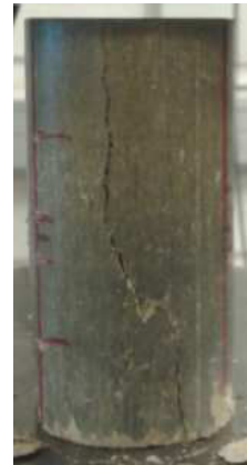
Fig. 8: Typical compressive failure mechanism (S10 – CS50 – W5.6)
