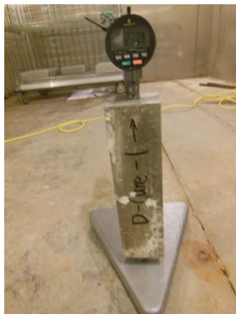
Figure 4 – Shrinkage test setup
