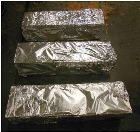
Figure 3 – Sealed concrete specimen
