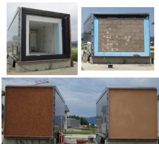
Fig. 3 : Photos of PASSYS cells – A: cell without tested wall – B: Cells with PIB Vicat hemp concrete – C: Cells with coated hemp concrete
