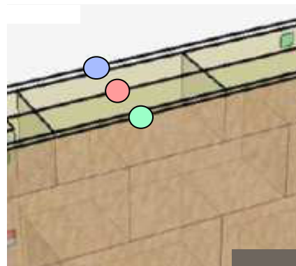
Fig. 4: Samples removed from PIB – 1: behind the interior coating - 2: at the middle of the block 3: behind the exterior coating
