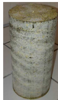
Fig. 2: Compacted specimen after casting [Tronet 14a].
